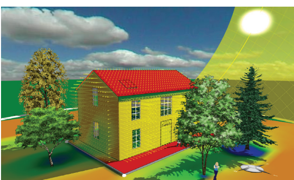
Figure 1. Solar analysis: The total solar radiation on a house in Boston on May 1 is visualized as a 3D heat map that reveals complex interplays among individual elements of a house and its surroundings.
