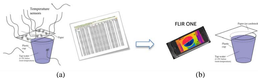
Figure 1. An example of how IR imaging empowers students to explore science more deeply through inquiry with an experiment that involves only a cup of water and a piece of paper. (a) Students use multiple temperature sensors to collect a lot of data for analysis with no guarantee to discover the thermal pattern shown on the screen of the IR camera on the right; (b) Students use an IR camera to instantly discover the thermal pattern, enabling them to conduct more follow-up investigations to dig deeply into the profound science that this seemingly trivial experiment actually reveals (Xie, 2012a).
