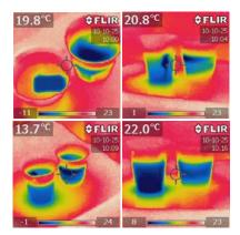
Figure 14: Seeing the thermohaline stratification. This experiment used just a cup of tap water, a cup of salt water, and some ice cubes. The two cups were placed next to each other on a table for comparison.
