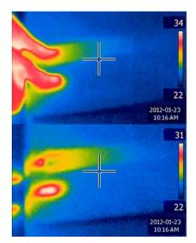
Figure 1: This experiment shows a comparison of thermal conductivities of metals and foams. A thin aluminum strip was placed on top of a foamcore board. They were covered up by a piece of paper to eliminate the effect of different emissivities of the metal and the foam. The two fingers were used as identical heaters. learning opportunities for students that have never been experienced in the classroom before.
