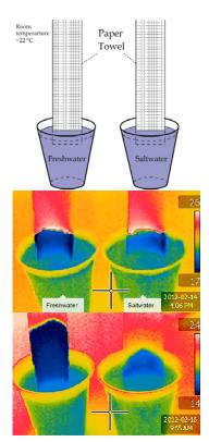
Figure 13: Capillary actions of freshwater and saltwater in two strips of paper towel caught by an IR camera. The upper thermogram was taken when the strips came into touch with water. The lower one was taken 18 hours later.
