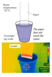
Figure 10: A piece of paper warmed up when it approached, but did not touch, water in a cup. caught a fire. Considering that water was cooler than the paper-due to the evaporative cooling effect-as shown in the thermogram, it appeared that heat were able to go against the temperature gradient and transfer from water to paper. We know heat cannot spontaneously flow from a cold object to a hot object. So what caused this strange phenomenon?
