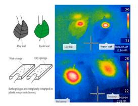
Figure 3: These two experiments compared the heat transfer from fingers to a dry leaf and a fresh leaf (upper) and to a wet sponge and a dry sponge (lower). It was shown that more heat transferred to a fresh leaf than to a dry one, and to a wet sponge than to a dry one, suggesting the role of water content on storing thermal energy.
