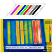
Figure 6: Comparing light absorption of different colors.
