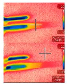
Figure 2: This experiment is approximately opposite to the one described in Figure 1. Thermography creates an illusion as if cold could also flow just like heat. In the upper thermogram, the two cold pieces were laid on the setup. In the lower one, they had been removed.
