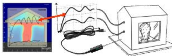
Figure 2. This illustration shows an example of data from a simulation being compared to lab data. The scale model house on the right generates temperature-time graphs near the ceiling and floor shown in the center. The temperatures at similar places generated by the computational fluid dynamics simulation on the left are sampled to generate comparable graphs, shown over the visualization. The simulation makes it obvious why the ceiling temperatures are so much higher and suggests other locations within the scale model house to measure. Students could determine whether there is a narrow rising column of hot air, whether it spreads out across the top, and where to place better insulation or fans.
